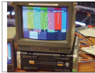
Figure 2.117 Graphics are an important part of today's productions. Here is a telestrator, used by the "color" announcer, the most notable being John Madden, to graphically diagram action. Here a technician has indicated that the telestrator is ready for use.
