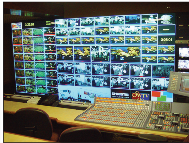
Figure 2.125 The monitor wall in the production compartment has required support on the part of the engineering staff for the last 20 years. Clients had to select which source would go to which monitor. Then truck engineers had to implement the decision and ensure that the monitor had tally when its source was selected for air. That used to be done via patching; now a lot of trucks use routers for at least a few monitors. This photo is of the latest wave of monitor walls. Instead of individual monitors, it is actually six rear projection monitors. Up to 16 sources can be displayed at once on each display, or just one if desired. The infrastructure that generates the displays also tallies the source, no matter where it is located on the display. This setup adds an additional layer to monitor wall setup, but makes for an extremely flexible wall for the client.
