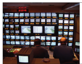
Figure 2.123 The monitor wall in the production compartment must not only have sources assigned to monitors, but many walls also have under-monitor tally displays. The monitor below the program monitor, labeled "Cam-2," is on-air, as indicated by the red display.
