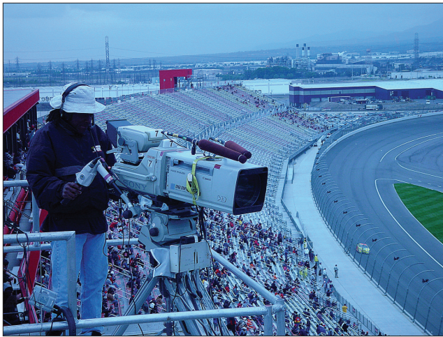
Figure 2.129 During the fax, camera operators will confirm that they have communications with the director and whomever else they need to talk with. They will also confirm that the tallies on their cameras are operating, and that they see return video from the truck. Return video is a program or some other video feed that they can select on their viewfinder. This return feed helps them frame their shot correctly when they are part of an effect.
