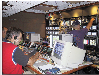
Figure 2.130 The tape compartment will confirm that any VTRs or servers expected to record can do so, and that all required playback devices work, and operate properly in slow motion. (Source: Core Digital Technologies/SWTV)
