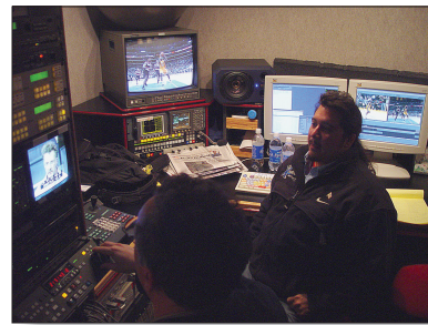
Figure 2.118 This is an edit bay in a utility trailer that is intended to allow for more complex editing to produce slick-looking tape packages. The editing bay also takes some of the pressure off the production unit's tape compartment. An edit bay typically includes a couple of VTRs. Often today that would be a VTR and a video server that also acts as an editor. When only VTRs were involved, one VTR would playback the raw material, and the second would be used to assemble a finished package. A separate editing controller controlled both VTRs. Today most video servers used in editing environments take over the role of the editing controller and control the playback VTR and other equipment in the bay.
