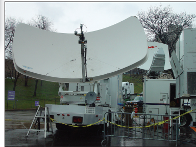
Figure 2.131 The large dish is the main C-band uplink. The smaller dish behind, mounted atop the truck, is the Ku-band backup feed.
